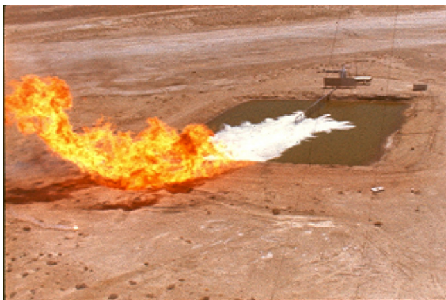
Plate 3. Vapor cloud fire in China Lake test. Fire held at pond' edge during flashback due the flame holder effect from the elevation difference between ground and water levels.
